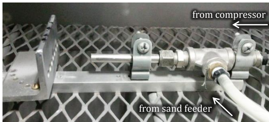
Figure 3.2 Configuration of nozzle and specimen holder
